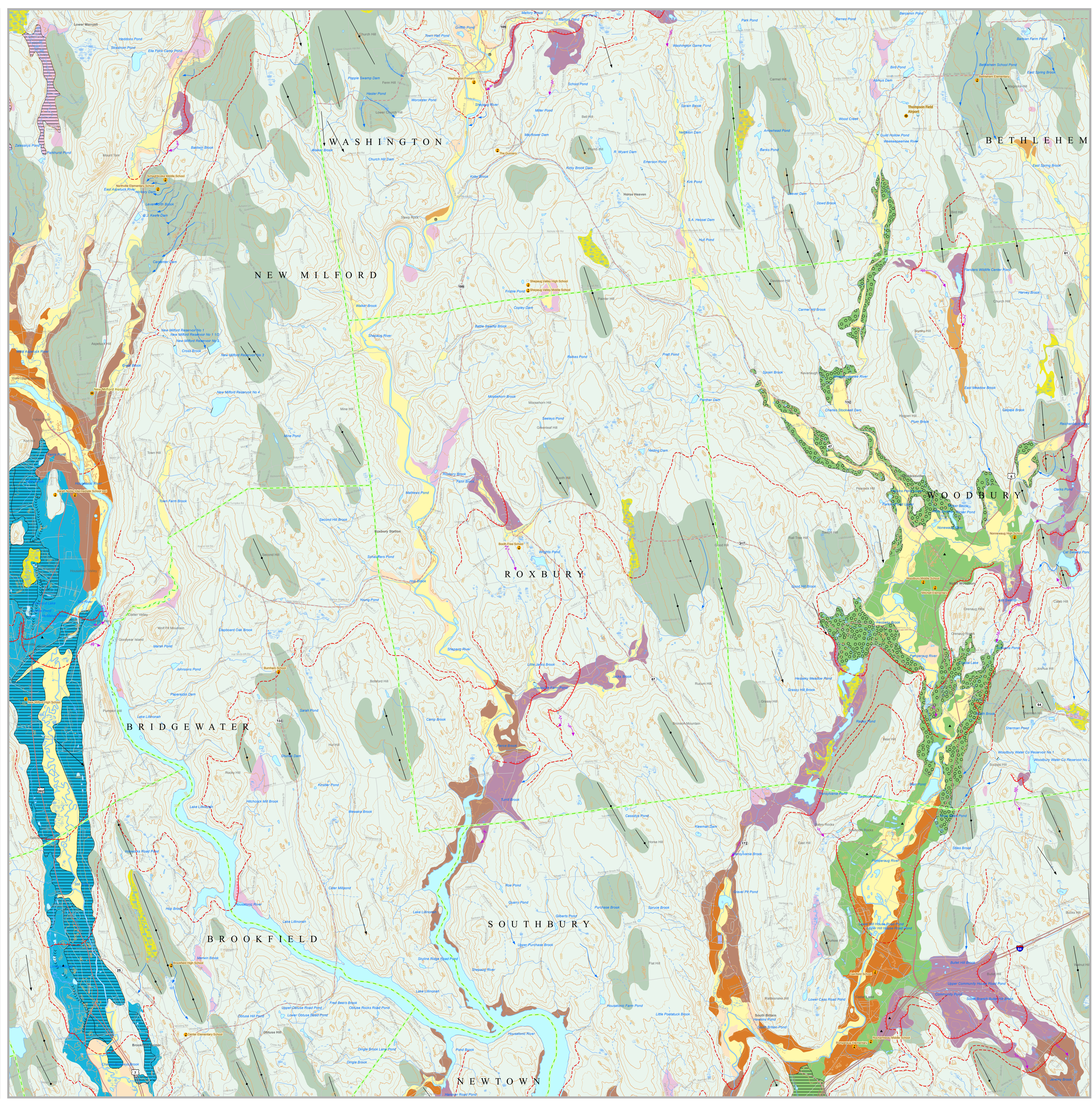
Figure 1: A morphosequence is a body of meltwater deposits composed of a continuum of land forms, grading from ice-contact forms (eskers, kames) to non-ice-contact forms (flat valley terrace, delta plains), that were deposited simultaneously at and beyond the margin of a glacier, graded to a specific base level. Grain-size decreases from coarse gravel at ice-contact, roads, through sand and gravel and sand beneath delta plains and forest slopes to silt and clay in lake-bottom deposits (after Stone and others, 2005).
