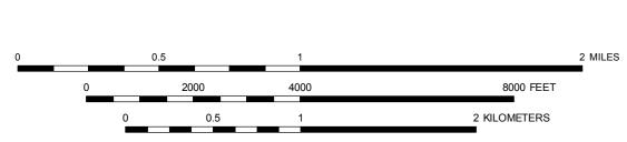
SCALE 1:24,000 when map is printed at original size (48 x 36 in) State Plane Coordinate System of 1983, Zone 3526 Lambert Conformal Conic Projection North American Datum of 1983
