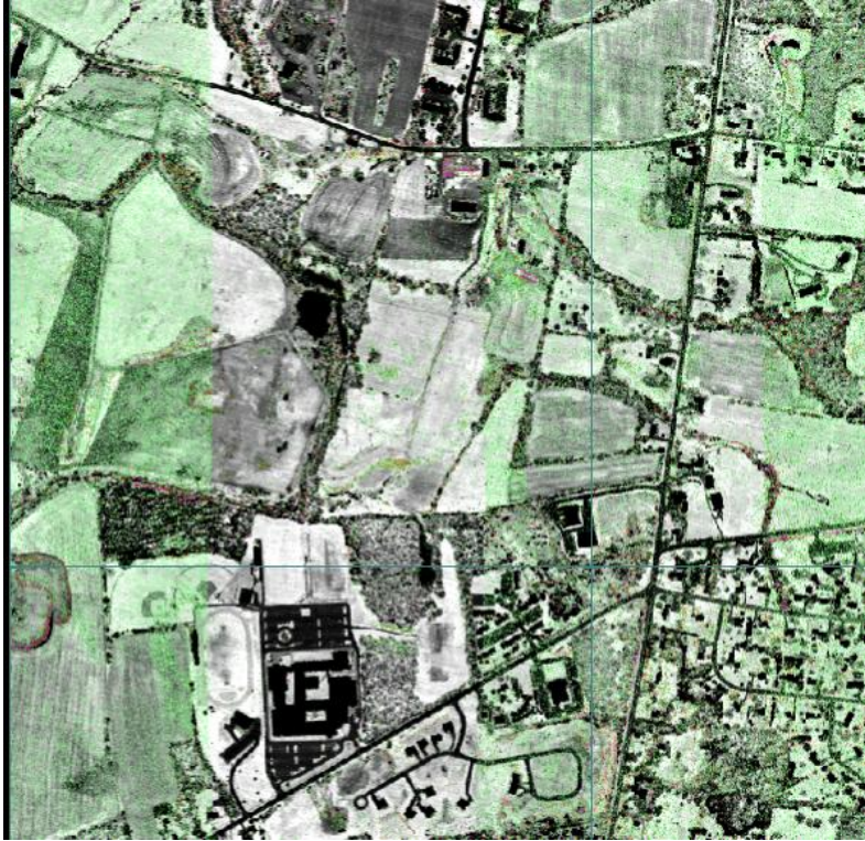
Figure 5: DZ orthos created from ground only points. Some red pixels are visible along embankments and sloped terrain, as expected. Open, flat areas are green indicating the calibration and relative accuracy of the data is acceptable.
