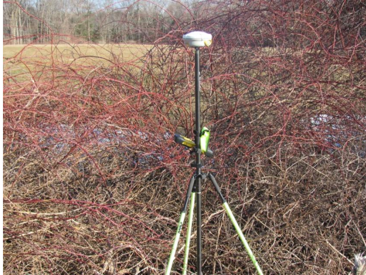
Figure 15: Survey Checkpoint GWC-4. This checkpoint is located in impenetrable brush that does not adequately give the LiDAR sensor a chance to measure the ground surface. Due to the poor placement of this checkpoint, it was not used during vertical accuracy testing.
